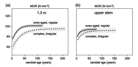
**Fig. 9** Relationship between strength (MOR) and cambial age in even-aged pure stands and uneven-aged pure stands of black spruce (Picea mariana (Mill.) B.S.P.) according to Torquato et al. (2014). The strength of timber from complex stands is lower at breast height (**a**) as well as in the top of the stem (**b**)
