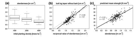
**Fig. 2** Slenderness as a proxy is affected by initial planting density (**a**) and affects sawn timber strength (**c**). The slenderness of a tree is transformable to the taper of logs (**b**). Tree slenderness is higher among low establishment spacing. Trees of high slenderness are characterised by high sawn timber strength (Rais 2015)
