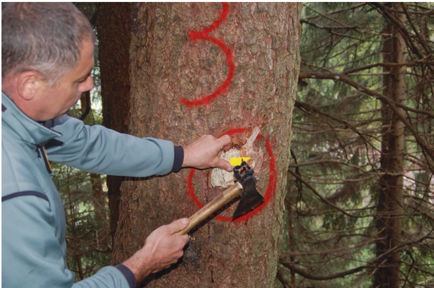
Fig. 9.3 Brand hammer used to mark trees. Note the area debarked with the sharp part of the tool and in the back of it the shape of the brand. Painting and yellow tags were part of a test and would not be used in common tree marking together with brand hammer
