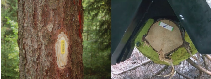
Fig. 9.9 On the left, an UHF RFID tag used to mark a standing tree, on the right an UHF RFID applied by the processor head after crosscutting
