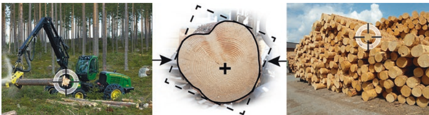
Fig. 9.8 Biometrics fingerprinting is based on the elaboration of visible and measurable characteristics of the log end, compressed in vector-format information. (Credit: Rudolf Schraml)
