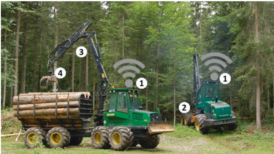
Fig. 9.2 Modern forest machines feature as a standard georeferencing sensor and wireless data transmission system (1) and encoders (in case of processor heads – 2). Additionally, accurate crane positioning systems (3) and grapple load cells (4) are increasingly used
