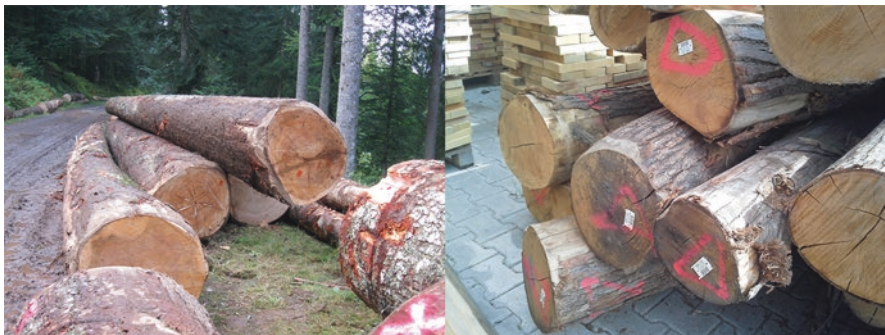
Fig. 9.5 On the left, logs recently hauled marked with plastic tags (orange). On the right, two models of plastic tags with numerical and UPC barcode
