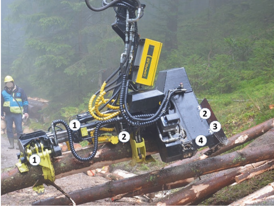
Fig. 9.13 Prototype of intelligent processor head equipped with sensors for timber quality assessment and tracking of logs
