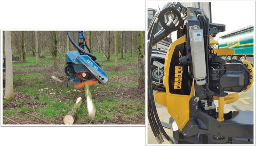
Fig. 9.4 On the left, a timber processor crosscutting a tree. Just after this operation, it is possible to mark the cut section with colors. On the right, a processor head equipped with color spray: the blue color tank is visible
