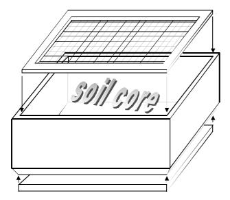
**Fig. 1.** Equipment for excavation of ECM. A steel frame with sharp lower rims for taking the soil core, a narrow-edged perspex frame stringed with a nylon grid of 10 mm width (above) for fixing the roots and ECM in their natural position, and a perspex plate (below) for preventing loss of soil.
