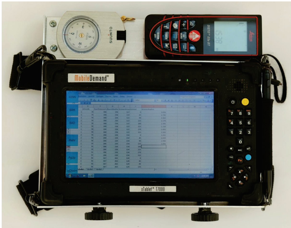
Fig. 4 Instrument composition which was used to measure the crown radius of the trees. The mobile tablet, the compass, and the laser distance meter are attached to an aluminum frame. The measured distances are sent by Bluetooth from the laser distance meter to the mobile tablet. The continuous alignment with the stem is done with the compass. The person who taking the measurements, can carry the instrument composition with an attached portable system.
