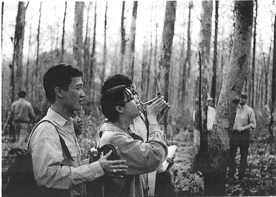
Fig. 1: Height measurement with a Blume-Leiss device on the Teak experimental plot no. 2, stand age 28 years, Maeh Moh plantation (Northern Thailand).
