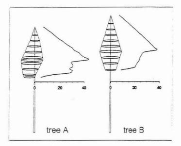
Diagram 2 : The diagram shows two trees and their branch diameter distribution. Tree A with an asymmetrical crown shape due to onesided competition and tree B with a fairly symmetric crown. Although the mean crown width of both trees is equal, tree A has significant larger branch diameters due to asymmetry. The branch diameter of tree A exceeds the critical 40 mm of the log-grading rule EN1927-1 for live branches in class B in Norway Spruce.
