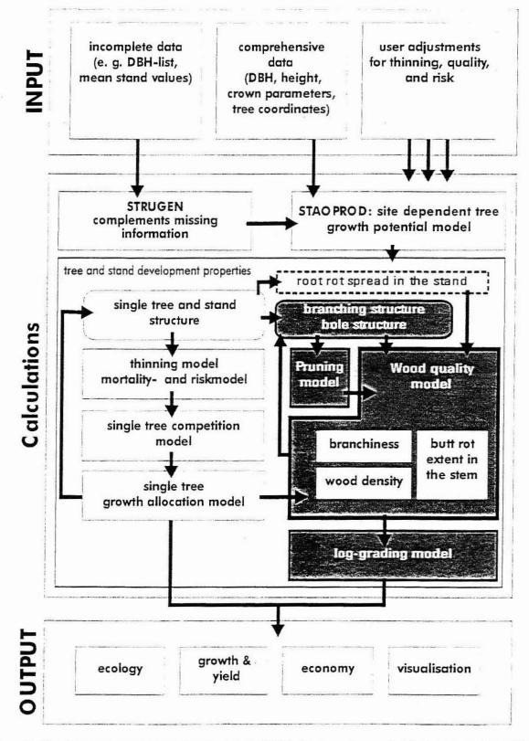
Figure 2 : The diagram shows the structure of original SILVA (white boxes) expanded for the root rot (dotted box) and wood quality model (dark grey boxes) and the interaction between the submodels.
