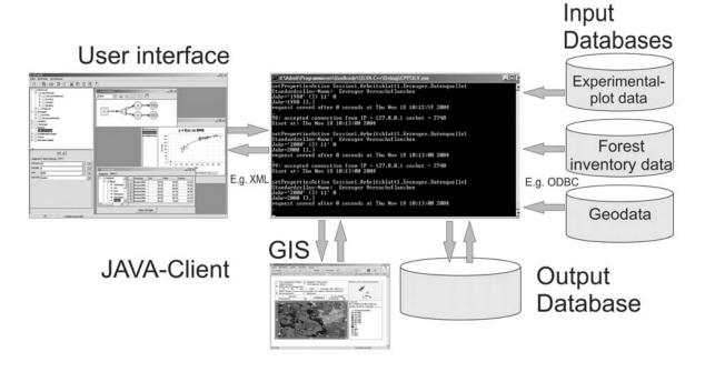
Fig. 9. Client-server solution for the management model SILVA 3.0: Main elements are the client with the user-interface, the server with the simulation model, the linkages to different data bases for the input of start values for simulation runs (e. g., inventory data, geo-data) and output of results (e. g., criteria and indicators of the system state).
